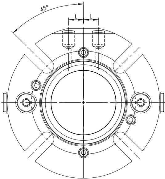
Max inside flush pressure = 12 bar
