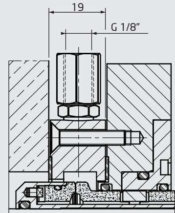
The axial built-in measurement increases with 19 mm irrespective of the shaft dimension.
