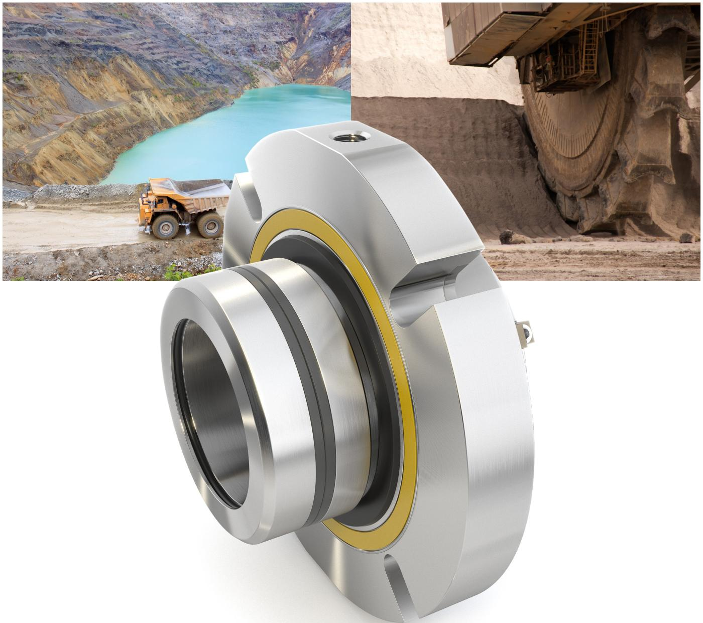
Huhnseal BFS is a balanced single mechanical seal specially designed for slurry applications. The spring package is placed outside of the product zone to avoid clogging. The use of this spring package allows for larger axial movement capabilities compared to conventional spring packages. The design is robust with premium materials from top suppliers. In the sealing area the surfaces are smooth with no sharp edges and corners to avoid inducing turbulent flow which will increase the wear.
